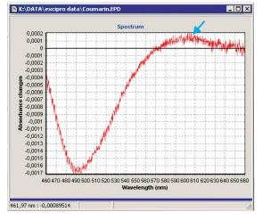
Transient absorption spectrum measured in Coumarin 30 dye solution with the multichannel detection at 460 nm - 660 nm. Blue arrow shows a peak of  $0.13 \pm 0.01 \text{ mOD}$  at 660 nm and demonstrates the Hatteras excellent sensitivity.
