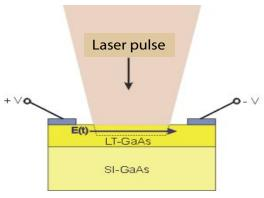
$\mathsf{A}$  short laser puls with puls width < 1 ps is focused between the electric contacts of the PCA. The photons of the laser pulse have a photon energy E = hv - h larger than the energy gap Eq and are absorbed in the film. Each absorbed photon creates a free electron in the conduction band and a hole in the valence band of the film and makes them for a short time electrical conducting until the carriers are recombined.
