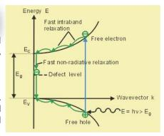
I o get the needed short carrier lifetime, the film must include crystal defects. These defects can be created by ion implantation after the film growth or alternatively by a low temperature growth. Low temperature grown GaAs (LT-GaAs) between 200 and 400 °C contains excess arsenic clusters. These clusters create defect levels within the band gap Eg and lead to a fast non-radiative recombination of the electron-hole pairs within a time interval < 1 ps.
