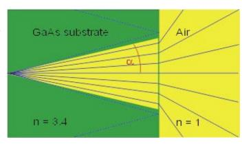
can escape the substrate. For GaAs with n=3.4 the escape solid angle is  $\Omega=0.28$ . This is only 4.4% of the forward directed
