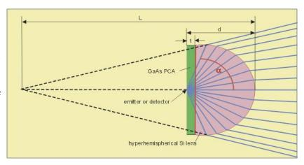
the hyperhemispherical lens is aplanatic, that means without spherical and coma aberration. For a silicon lens with almost the same refractive index  $n \sim 3.4$  as GaAs at therahertz frequencies the distance is d = 1.29 r with the lens radius r. The height h of the aplanatic hyperhemispherical lens is therefore h = d - t with the thickness t of the semiconductor PCA.
