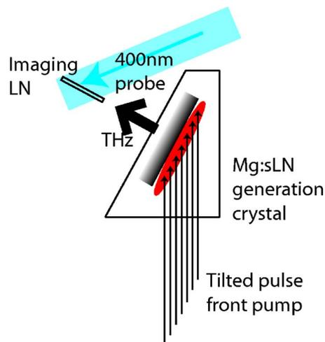
FIG. 1. (Color online) Experimental geometry for the generation and detection of terahertz radiation.
