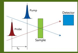
For time resolved pump-probe experiments two independently tunable and synchronized pulses are needed.
